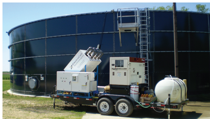
Figure 1 This self-powered, BioElectric treatment system can be delivered by a pickup truck, set up in hours and it will process up to 6,000 gallons per hour unattended 24X7.
