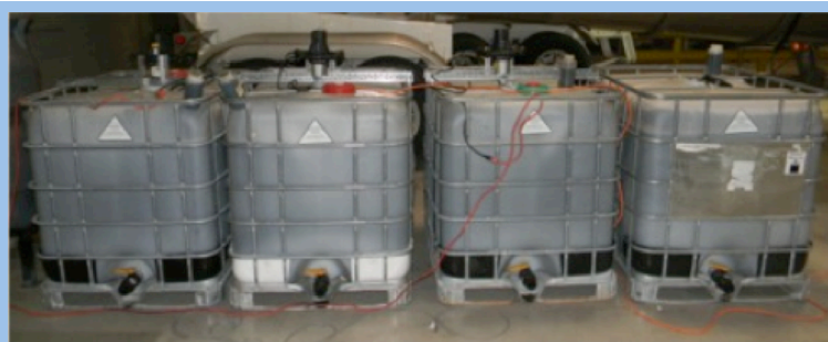
Figure 4. Four of the six totes used in the pilot. Three of the totes were mixed using modified, low speed drywall mixers configured to keep material moving without inducing aeration.
